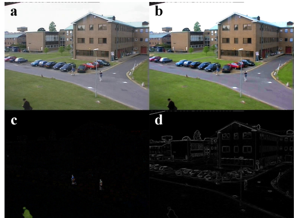
Figure 1. Inputs of the subsequent UMM's cores: a – input image [PETS01a], b – color core input, c – difference core input, d – gradient core input.
